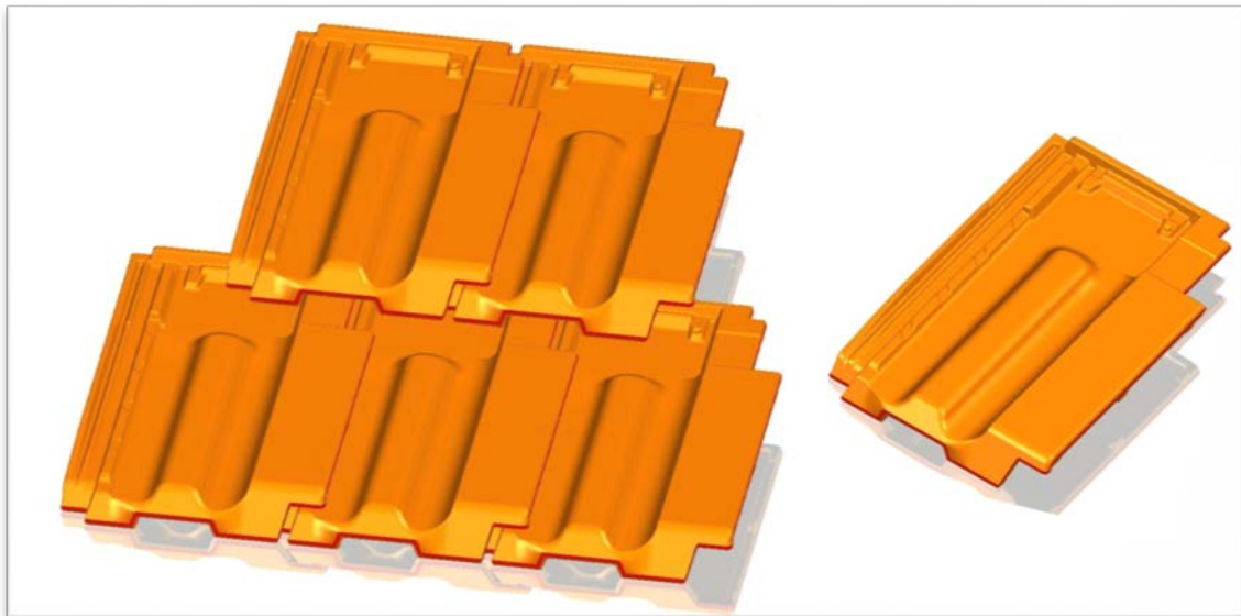
Fig. 1. Modeling and assembly testing of the Marseillaise tile project.
