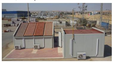
compared analysis on the two mock-ups in Ferrara (ITALY) and Yerucham (ISRAEL) are carrying on. These data are the basis to realize the computing program **SENSAPIRO** (Software Energy SAvings PItched Roofs), property of ANDIL. The program
