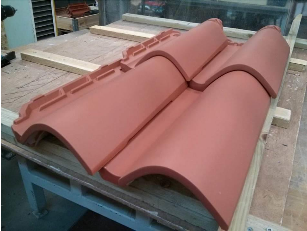
A Portoghese roof tile prototype. Image courtesy of Monier Technical Centre GmbH.
