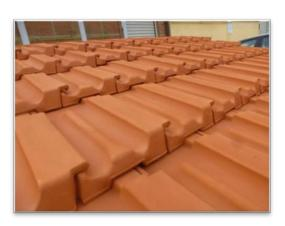
We have designed a new shape of Marseilles tile, characterized by a high permeability, by a perfect overlapping and by a better energy performance of the underlying covering, through the reduction of the passive influence of solar light, which determines the improvement of the above sheathing ventilation. The new tiles, produced in our production lines, have been placed in the real-scale pilot building of Cadelbosco (RE). In the
